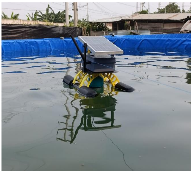
Figure 6. Testing of the buoy prototype in a real aquatic environment
