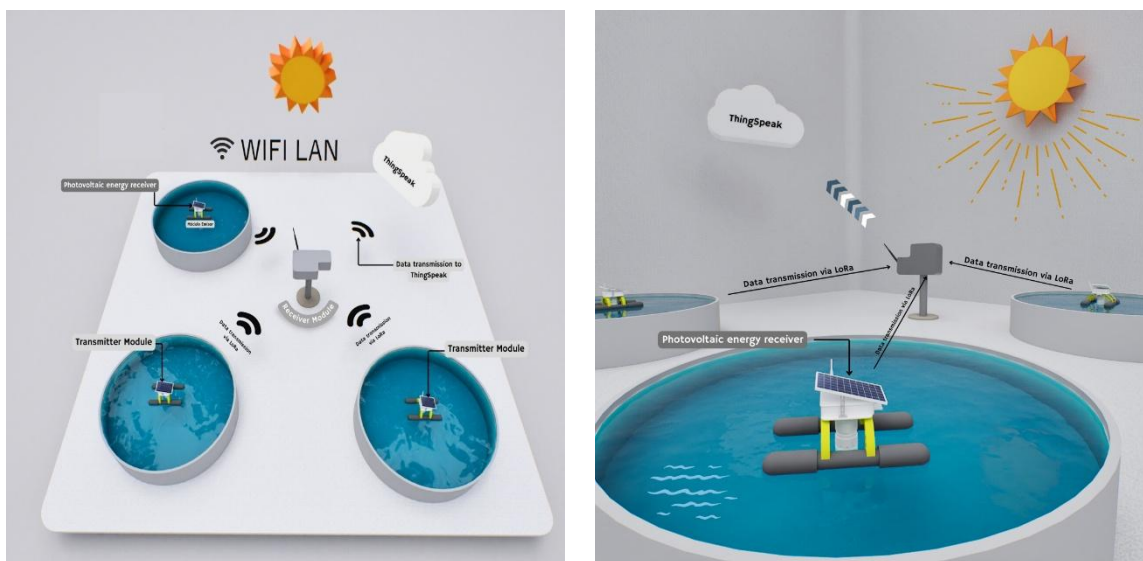
Figure 5. Conceptual design for sending data to the cloud
