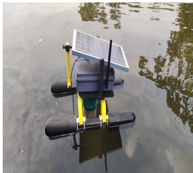
Figure 6. Testing of the buoy prototype in a real aquatic environment
